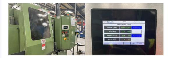
A £30K Variable Speed AC Drive upgrade project replaces an existing troublesome obsolete control system, resulting in reduced downtime and supporting increased production and reduced downtime on the Pneumatic Components Ltd Wickman C&M Machine Auto Multi in Sheffield.
